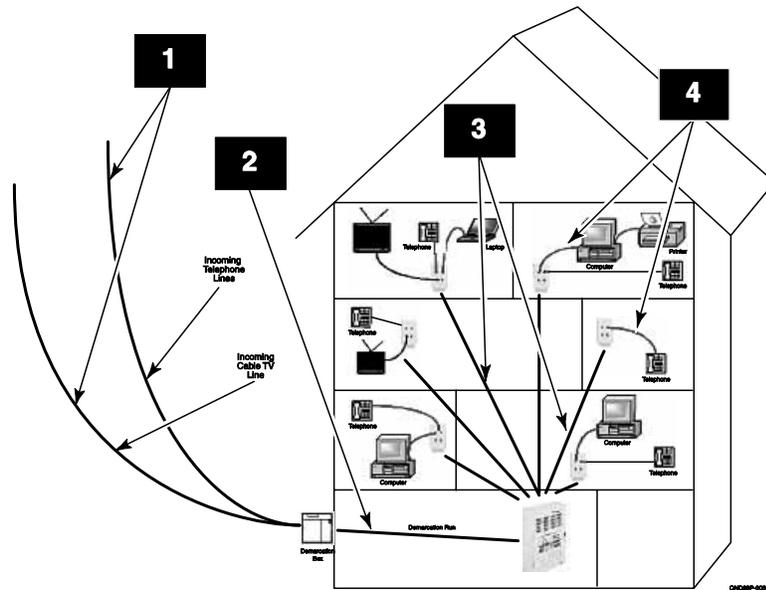
2. Once these signals and services are connected to the Demarcation Box, a Multi-Media cable is used to connect the Demarcation box to the Distribution Panel. This is referred to as the Demarcation run.
